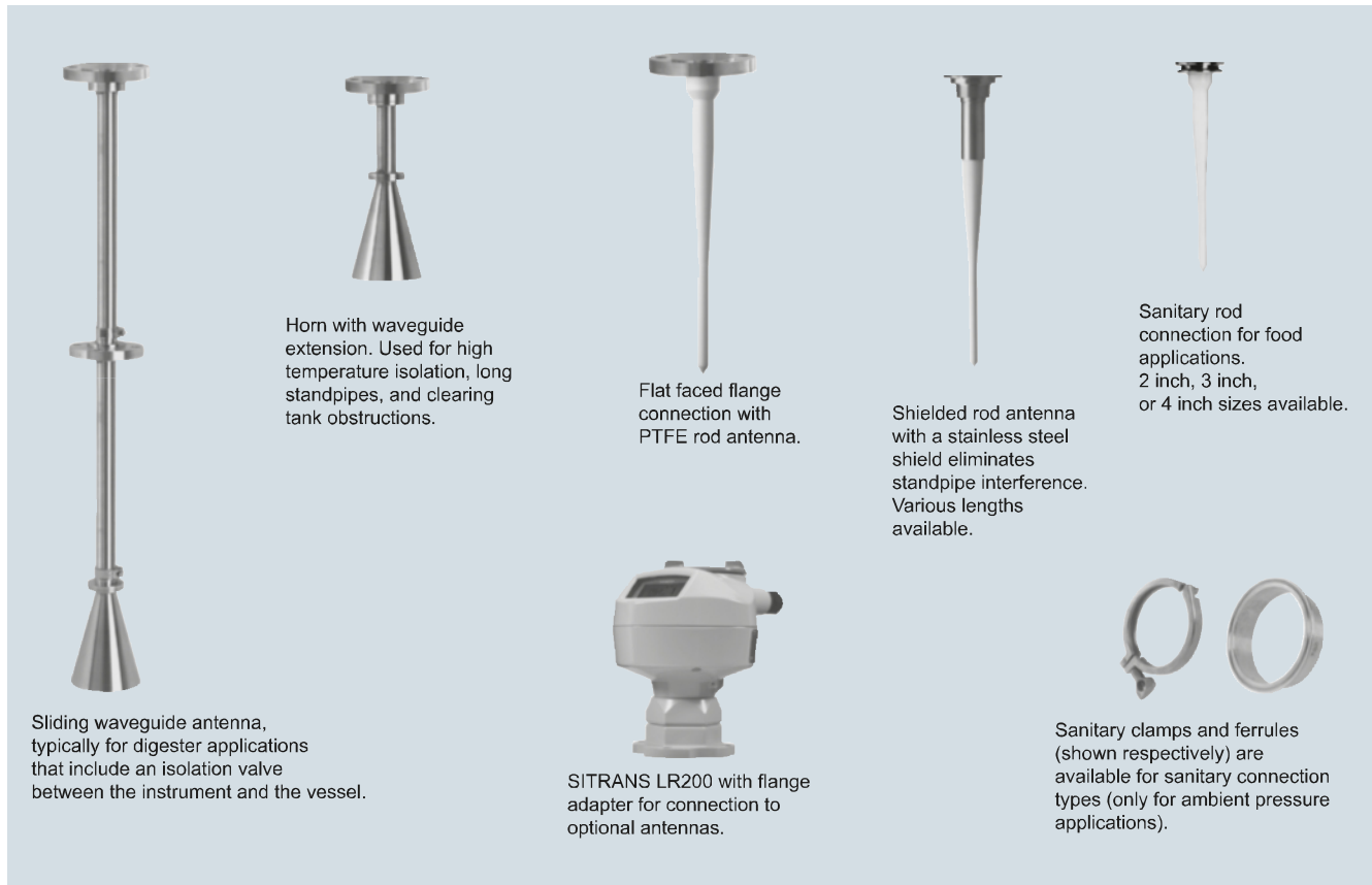
Antenna configurations for SITRANS LR200
